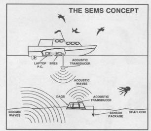
DIAGRAM SHOWS essential components of SEMS III. Abbreviations and their meaning: P.C. — personal computer; BRES — Buoy Repeater System; DAGS — Data Gathering System
